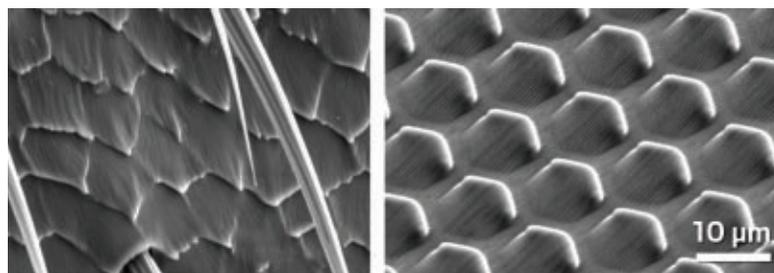
Tiled microstructures on a firefly lantern (left) make it shine brighter. The man-made mimic (right) has the same effect.
